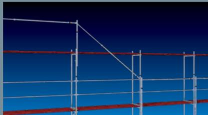
To create a preceding guardrail system, the guardrail posts are raised upwards across all bays of a level; the telescopic guardrail automatically follows.
