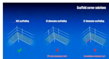
The advantages of the metric solution become most evident whenever corner constructions are involved: no odd-looking values, no improvisation with coupled tubes. The bottom line is that even less material is needed.
