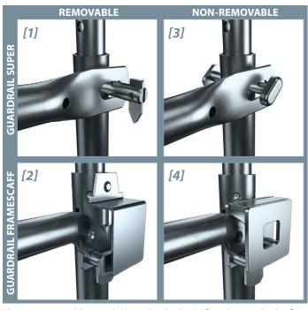
The non-removable guardrails are hooked in before the standard is fitted. When the standard is set upright, the toggle and guardrail opening twist against each other so that removal is no longer possible when the standard has been mounted.
