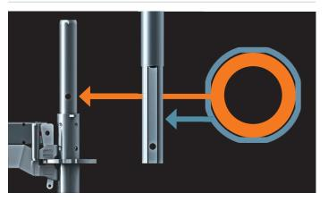
Due to the standard dimensions for standard and tube connector diameters, the combination with conventional systems is possible. The optimised, reduced wall thickness of the SUPER-RS standards is compensated for by compressed lower tube ends.
